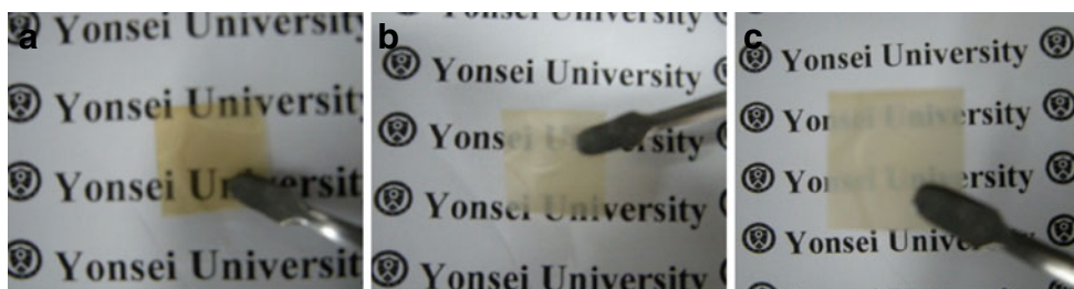
Fig. 1 Photographs of P(VDF-co-CTFE)-g-PSSA/SiO 2 -SO 3 H nanocomposite membranes; MPTMS content is a 5 wt.%, b 10 wt.%, and c 20 wt.%
